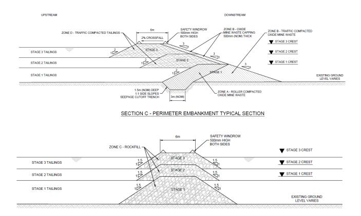
SECTION B - DECANT ACCESSWAY TYPICAL SECTION
