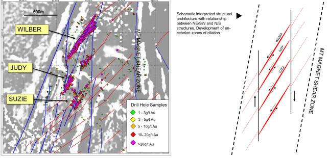
Figure 23 – Drill sample assay locations coloured by grade, overlain on 2nd Vertical Derivative aeromagnetic image including a simplified overview of the shear structures.
