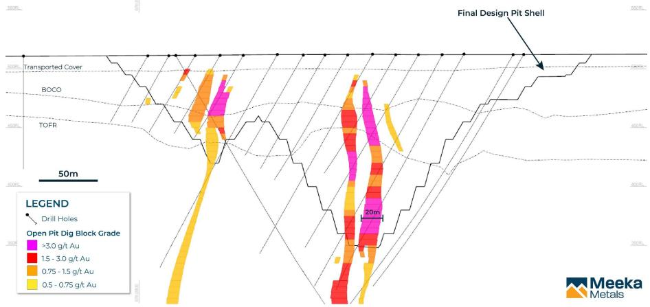
Figure 39 – Cross section at Turnberry Central showing dig blocks and final pit limits, 7087550N.
