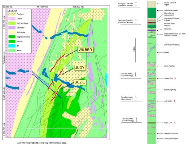
Figure 21 – Andy Well interpreted geology and mineralisation.
