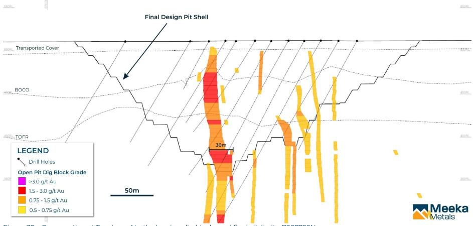
Figure 38 – Cross section at Turnberry North showing dig blocks and final pit limits, 7087795N.
