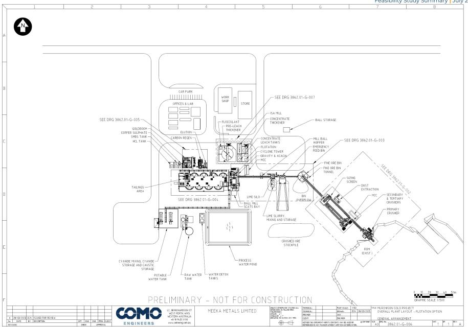
Figure 52 – 1.0 Mtpa CIL process plant layout.
