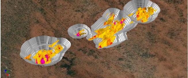
Figure 35 – Isometric view showing Turnberry final pit design shell and dig blocks.
