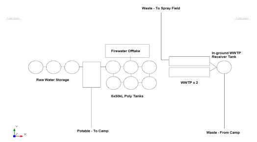
Figure 62 – Potable water and wastewater infrastructure layout.
