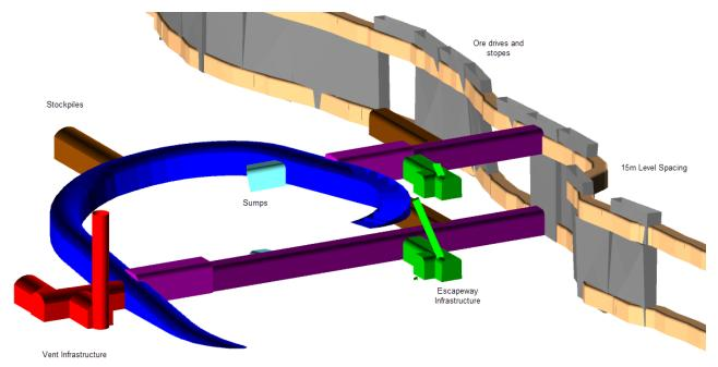
Figure 46 - Isometric view showing typical Andy Well level layout.
