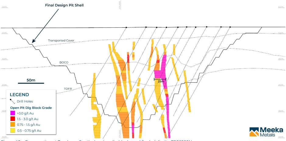
Figure 40 – Cross section at Turnberry South showing dig blocks and final pit limits, 7086560N.
