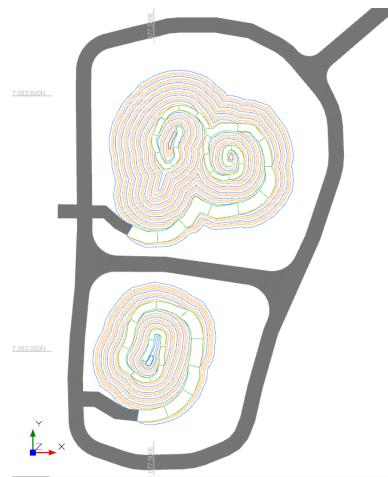
Figure 41 – Plan showing open pit design for St Anne's (design pit shell = Ore Reserve pit shell).
