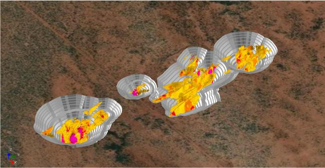
Figure 8 – Isometric view showing Turnberry final pit design shell and dig blocks.
