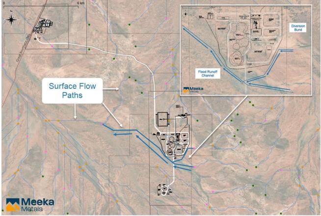
Figure 29 – Flood runoff model and diversion bunding.
