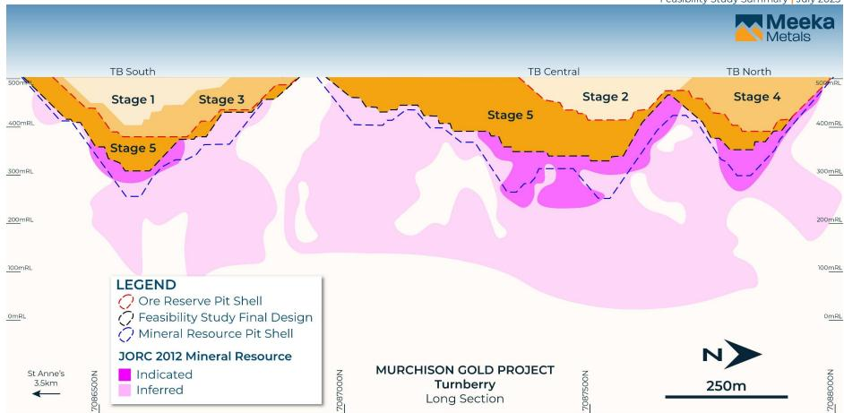
Figure 36 – Long Section showing open pit staging at Turnberry.
