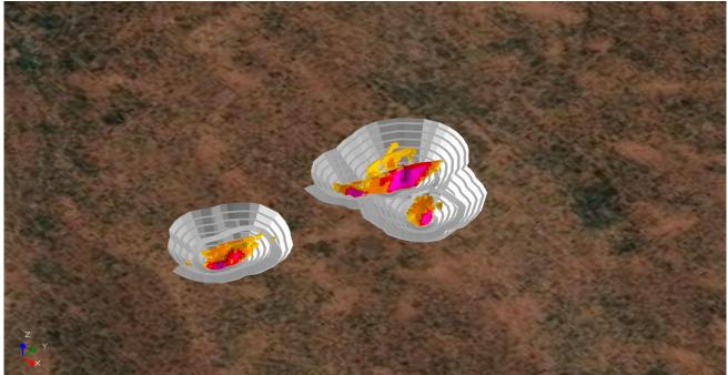
Figure 11 – Isometric view showing St Annes final pit design shell and dig blocks.
