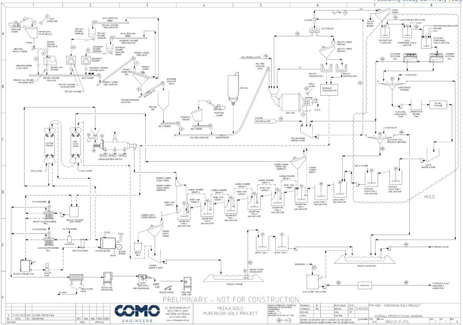
Figure 53 – 1.0Mtpa CIL plant flow sheet.
