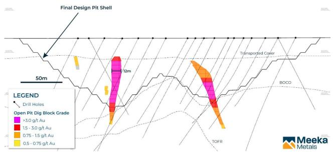
Figure 12 – Cross section at St Anne's showing dig blocks and final pit limits, 7083480N.
