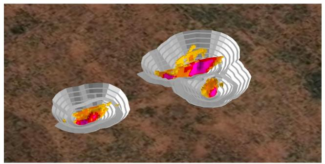
Figure 42 – Isometric view showing St Anne's final pit design shell and dig blocks.
