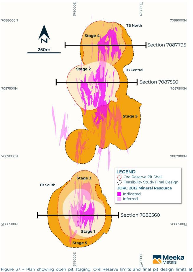
Figure 37 – Plan showing open pit staging, Ore Reserve limits and final pit design lin Turnberry.
